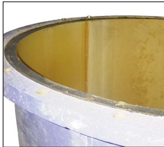
Polyisoprene lined casing - after use
