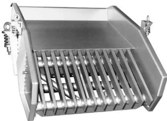
Model 85B Grizzly to de-lump iron ore.
