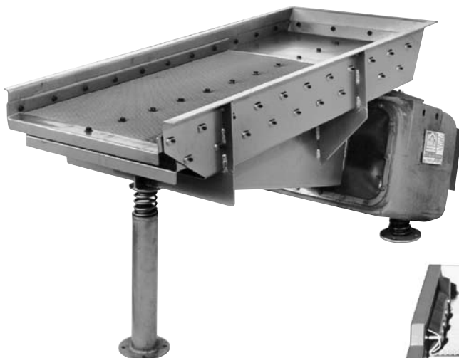
Model 52A with a stepped screen mounted on a portable cart.
